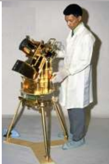
George Carruthers examine the gold-plated Lunar Surface Ultraviolet Camera prior to the Apollo 16 mission
